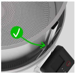
Once the sparge has finished, refit the lifting bar to the grain basket to lift and remove the basket from the boiler.
